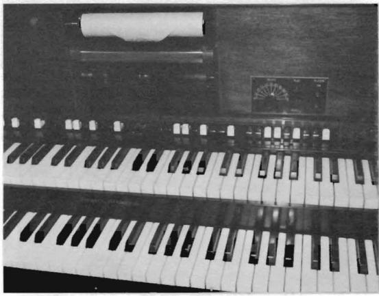
Note the roll mechanism and tempo regulator above the top organ manual.
