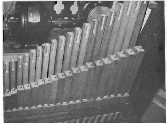
The pipework: Stopped flutes in the foreground and violin pipes in the rear.
