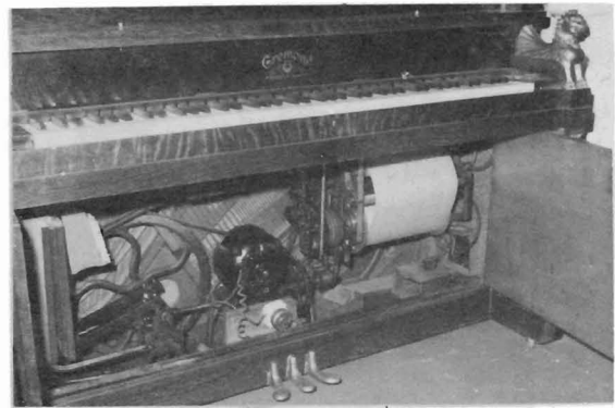
The roll drive and pump mechanism of the J.
