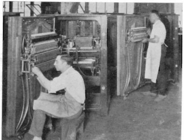
Mills factory scene: regulating the Violano piano action was one of the final steps.
