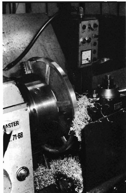
The large diameter pump pulley casting being turned in a lathe.
