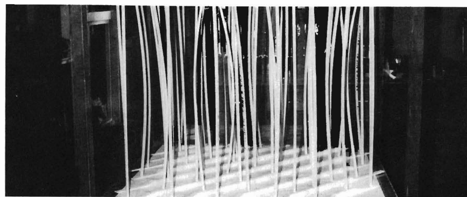
This hold-down jig presses the ribs to the soundboard until the glue dries.
