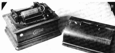
EDISON STANDARD , two-minute, dirty mechanism, but working. No horn, no reproducer, no crank. The case appears to have a new Edison decal.
