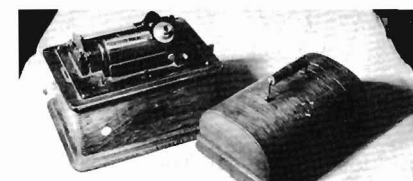
EDISON STANDARD , two-minute, oak case stripped and revarnished. Most of the original decal was saved. Mechanism is dirty and not working. No horn, no crank, reproducer lead screw follower is missing, as is the cover for the gear drive.
