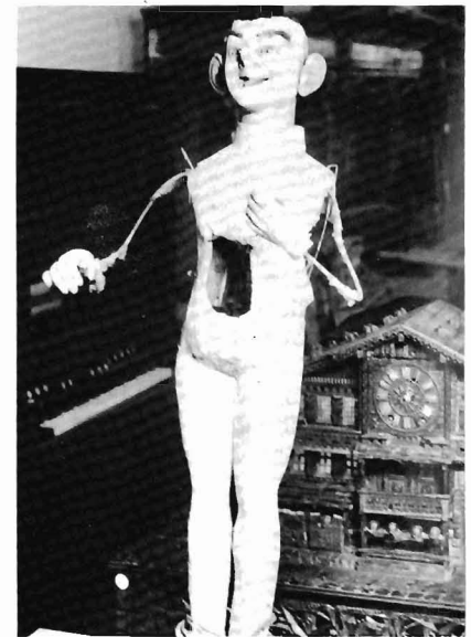
AUTOMATON , undressed, 36" high, with a partial clockwork mechanism in the center of the body, and a Mills Violarm electric bow motor in the base. Your move.
