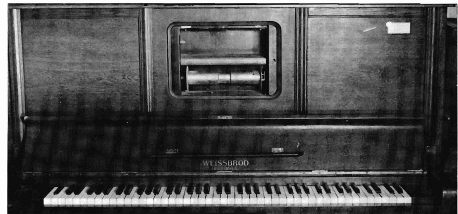
R. WEISSBROD EUFONIA UPRIGHT , serial number 20341. Case: oak. Finish: open grain. Ivories: perfect. Hammers: original. There is no evidence of prior rebuilding. The lower half of the bass side of the piano is missing veneer. The lower base strut needs repair. The electric pump drive motor is missing, as are some of its associated linkages. The piano
