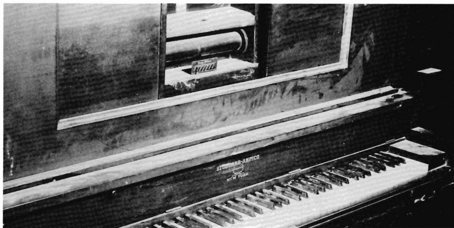
STODDARD AMPICO , serial number 40176, made between 1915-1919. Case: mahogany. Finish: alligatored. Ivories: original, many missing. Hammers: original. There is no evidence of prior rebuilding. During the years of World War I this was the type of
