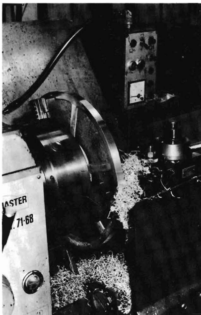
The large diameter pump pulley casting being turned in a lathe.
