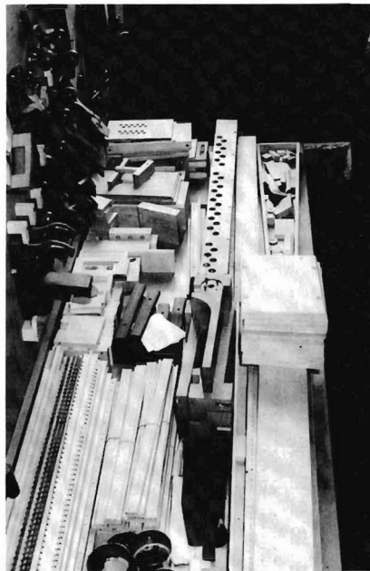
Precut parts for the pneumatic mechanisms ready for assembly.
