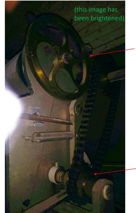
Large gear connects to the long drive shaft
