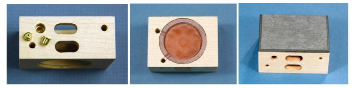
While the hole for the bleed cup was still damp with shellac, use a pin punch to tap the bleed in place. After gluing in the pouch assembly, I used a sharp chisel to cut a V-groove between the two face holes and the pouch on the pouch side of the valve. This provides air channels from these holes to the back of the pouch.
