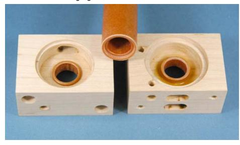
I pressed the lower seats into the block with a piece of <sup>3</sup>/<sub>4</sub>" diameter Bakelite tubing. I cut a shoulder on the inside of the tube 1/16" deep and with a diameter just larger than the 5/8" seat outside diameter. I used this as a tool to press the seat in until the tool was flush with the floor of the valve block, making the seat stick up 1/16" from the floor.
