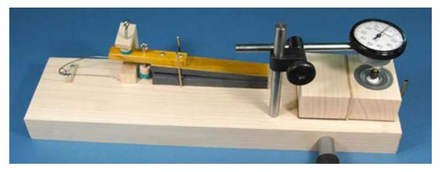
Here is the setup I used to test and adjust the valves. The test pneumatic is made to the specs of the 105, including the pneumatic movement adjustments and the pallet spring. I used a dial indicator for setting the valve travel with a rod mounted in the base to mount it over the valve. I used a quick release clamp to hold the valve during the test/adjust process.
