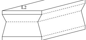
The force pressing on the top surface is:  $P \ge L1 \ge 2.181 \ge 1.875 \ge 1.636 \ Lb \ge 5$  "water gauge (WG). The force development due to the pneumatic cloth is similar to that developed on the wood. However, this sideways developed force acts to pull the moving board closed through the angle between the cloth and the board. This reduces as the pneumatic closes. When the pneumatic is fully **closed**, the force developed due to the cloth is zero.
