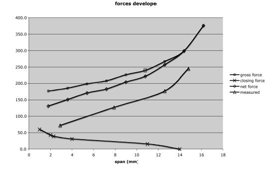
The measured force shows some discrepancy with the calculated value. What is confirmed is the higher developed force when the pneumatic is open compared to that when closed. These data are taken at a vacuum level of 5 inches. The data also shows the increasing closing resistance force as the pneumatic closes. The closing resistance force is a significant proportion of the total developed force measured at a percent opening of 10%. (around two to three mm)
