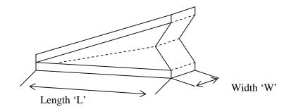
Force due to the wood, calculated at the moving end is:  $F_{wood}$ = (P x W x L) / 2 P is the pressure as before, and at 5" water gauge  $F_{wood}$  = (0.181 x W x L)/2 Lb force
