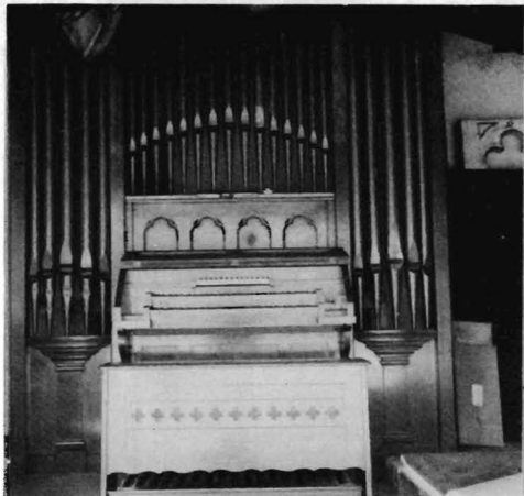
No.1. Circa 1908 tubular pneumatic Estey pipe organ (not automatic). Mostly rebuilt. Many ranks of pipes. Self contained. The main case with the pipework is about 10'6" high, 8' wide and 5'6" deep. The bench and pedalboard add more depth. With two 61-note manuals and 30 note pedalboard. 4" wind pressure. Nine ranks 4' to 16'. Beautifully finished light golden oak case. Originally used in a theological seminary.
