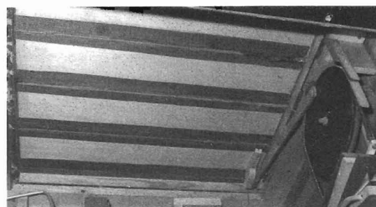
The swell shutters as seen from inside the instrument. These provide a fantastic degree of expression to the music.
