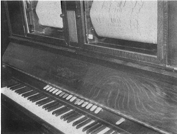
The 88-note rolls go on the left tracker, the 134-key orchestration rolls on the right side.
