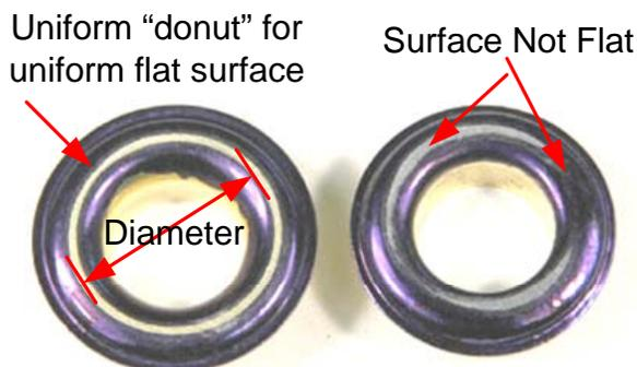
Some grommets do not provide a flat uniform surface and therefore do not seat and seal well. In fact they can fail miserably. As a quick check, rub one of the grommet faces a few times on a sheet of very fine emery paper glued to a flat surface. Look at the area polished into the surface to make sure that you see a uniform “donut” shaped area with no breaks.
