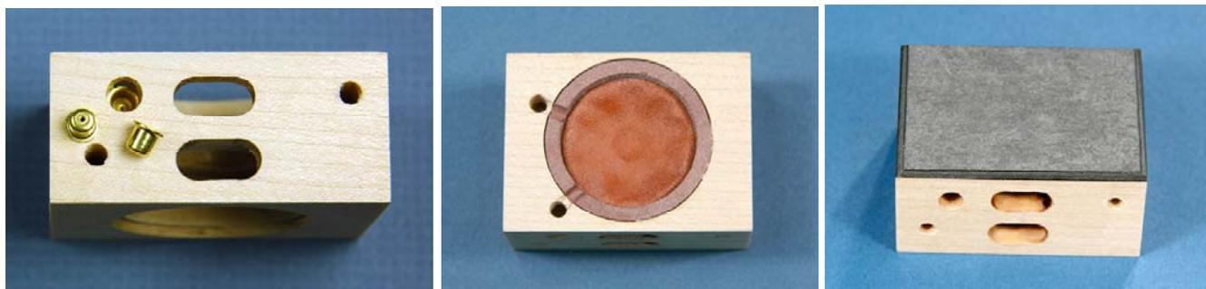
While the hole for the bleed cup was still damp with shellac, use a pin punch to tap the bleed in place. After gluing in the pouch assembly, I used a sharp chisel to cut a V-groove between the two face holes and the pouch on the pouch side of the valve. This provides air channels from these holes to the back of the pouch.
