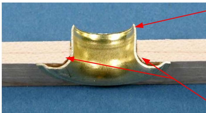
Some of the grommets narrow considerably at the neck and need to be trimmed. This section of the grommet needs to be ground away, down to the straight walled section of the the grommet opening. Also, you will have to make sure there are no burrs to catch the fluted stem. The valve floor will have to be counter-sunk so that the grommet will seat on the floor of the valve chamber.
