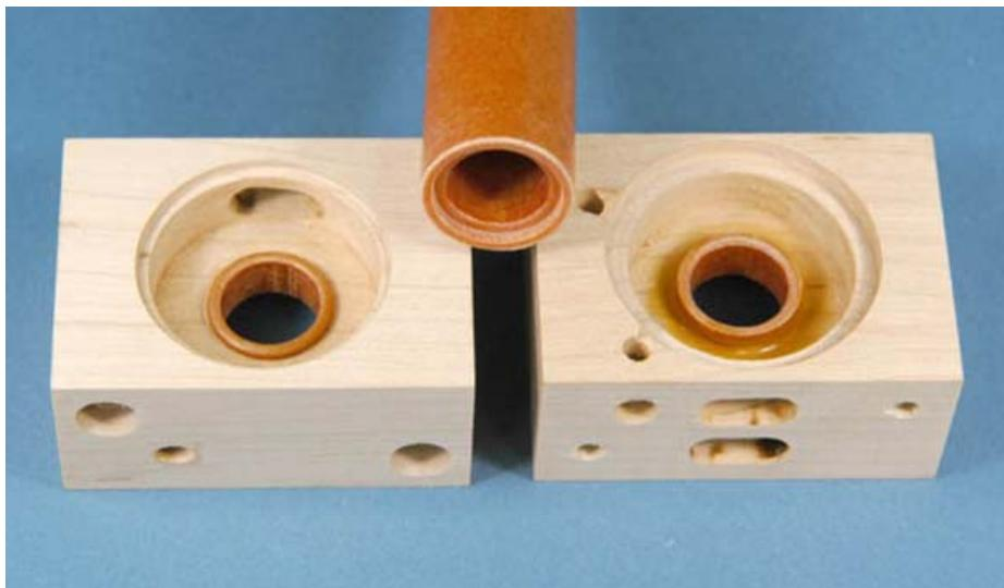
I pressed the lower seats into the block with a piece of  $\frac{3}{4}$ " diameter Bakelite tubing. I cut a shoulder on the inside of the tube  $\frac{1}{16}$ " deep and with a diameter just larger than the  $\frac{5}{8}$ " seat outside diameter. I used this as a tool to press the seat in until the tool was flush with the floor of the valve block, making the seat stick up  $\frac{1}{16}$ " from the floor.
