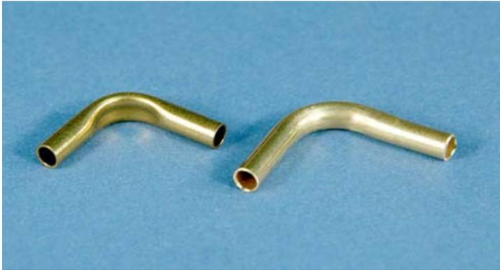
Over the years I have used tracker tube elbows from a supplier whose product looks like they were made by just bending and kinking the tube over the corner of a bench. Although it is true that the channel inside these tubes are sufficiently large to work ok, they look like the devil. And they obviously do not look anything like the original.
