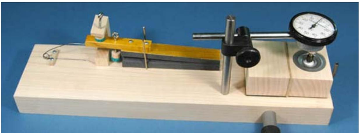
Here is the setup I used to test and adjust the valves. The test pneumatic is made to the specs of the 105, including the pneumatic movement adjustments and the pallet spring. I used a dial indicator for setting the valve travel with a rod mounted in the base to mount it over the valve. I used a quick release clamp to hold the valve during the test/adjust process.
